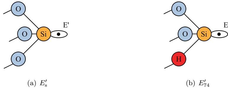
**Figure 3.7:** Possible configurations of an  $E'$  oxide trapping center as found in amorphous  $\text{SiO}_2$ . It comprises of an unpaired electron localized on a silicon atom which is back-bonded to either three oxygen atoms (a) or two oxygen and one hydrogen atoms (b).
