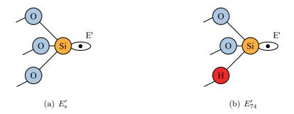
Figure 3.7: Possible configurations of an E' oxide trapping center as found in amorphous  $SiO_2$ . It comprises of an unpaired electron localized on a silicon atom which is back-bonded to either three oxygen atoms (a) or two oxygen and one hydrogen atoms (b).
